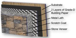
Then attach galvanized expanded metal lath to the substrate by nailing or stapling every six inches vertically and horizontally. The galvanized nails or staples should penetrate the studs a minimum of 1 inch. The lath should extend sixteen inches around corners.
